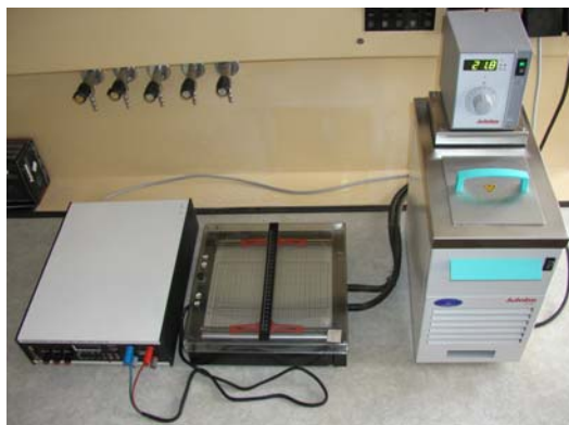
Figure 2. Technical equipment for isoelectric focusing is comprised of (from left to right) Electrophoresis Constant Power Supply EPSC 3000/150, electrophoresis unit Flat Bed Apparatus FBE-3000, cooling unit Julabo F12. Instead of cooling unit is possible to use cold water from draw-off tap. The next necessary equipment for preparing of gel is fume-hood and a rotating shaker for silver-staining of the gel.
